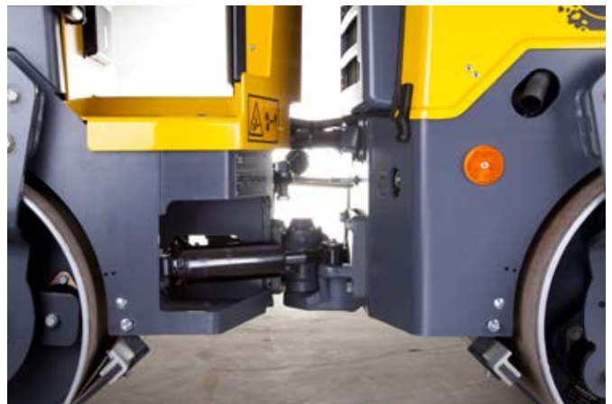
Long service intervals together with maintenance free steering hitch and steering cylinder contribute to a minimum of maintenance.
