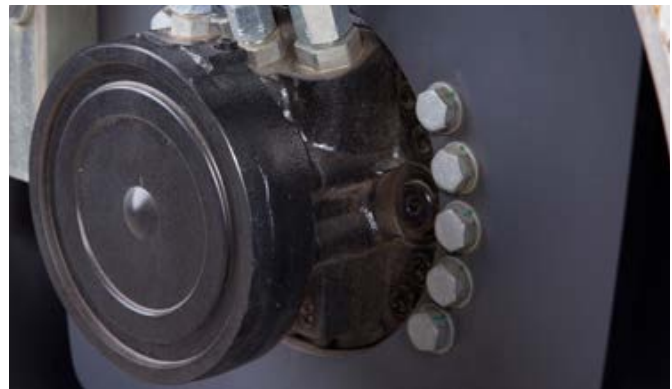
Fail safe brakes on both drums (or drum + combi wheels) which apply automatically in the event of failure in engine, hydraulics or electrical fault in the brake system.
