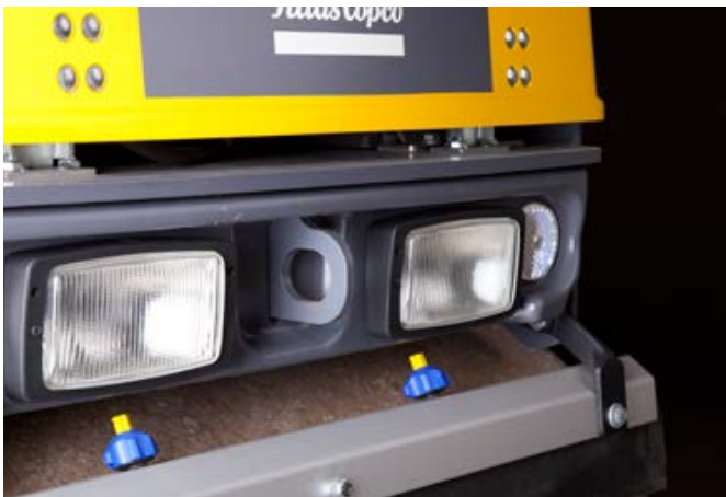
Pressurized sprinker system with a powerful water pump and with self draining sprinker tubes and nozzles.
